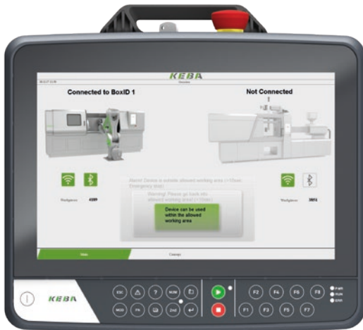
T155 with standard keyboard emergency stop twin circuit
