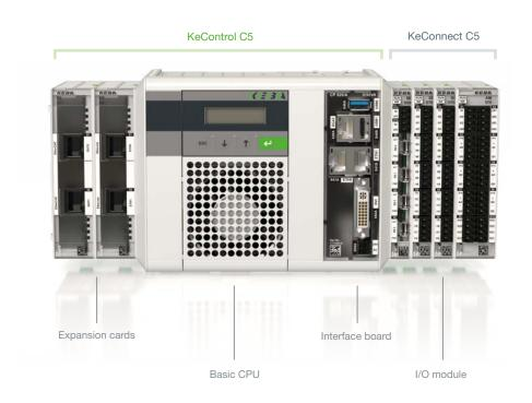
KeControl C5 complements the KEBA control family with high-performance compact controls that stand out for their consistent modular design. The KeConnect C5 I/O modules that can be connected on the right and the KeConnect C5 expansion cards that can be plugged in on the left provide customers with maximum flexibility in the configuration of their individual automation systems.
