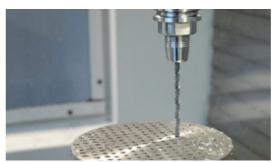
Vibration-assisted 6D drilling with magnetic bearing spindles has brought about a completely new drilling process, resulting in shorter chips and fewer burrs as well as increased process speed and drill hole quality. The integrated sensor technology also enables intelligent process control with material detection.
