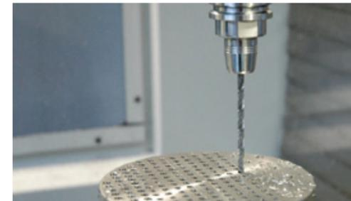
Vibration-assisted 6D drilling with magnetic bearing spindles has brought about a completely new drilling process, resulting in shorter chips and fewer burrs as well as increased process speed and drill hole quality. The integrated sensor technology also enables intelligent process control with material detection.
