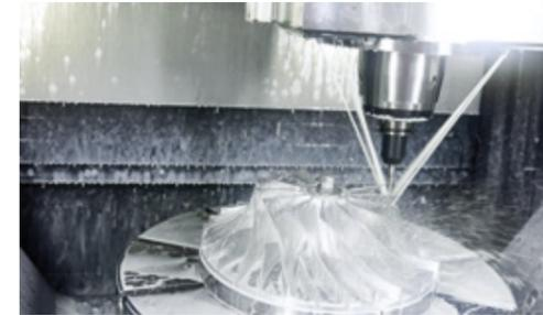
Grinding and high-speed grinding processes require extremely precise and flexible solutions. KEBA therefore offers the automation solution with Piko interpolation, block time 100  $\mu$ s, 50,000 blocks Look Ahead and programming language Lua, that provides our customers with their unique selling proposition.
